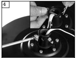
Remove keeper from pin. (see inset) Loosen the 2 set screws in yoke for downrod to slip into yoke.
