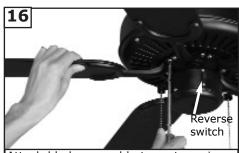
Attach blade assembly to motor using the motor screws and washers provided. Tighten screws securely. Setting the reverse switch in the down position will result in downward airflow and setting the switch in the up position will result in upward airflow.
