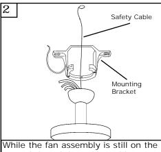
While the fan assembly is still on the ground thread the safety cable through the mounting bracket.
