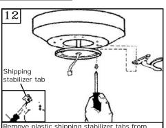
Remove plastic shipping stabilizer tabs from motor, if present. The screws, washers and motor pads are pre-installed to the blade holders. Attach blade assembly to motor by tightening first screw one turn, then tighten second screw securely. Then, go back and tighten first screw securely.
