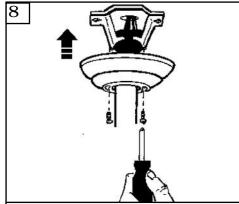
Raise the canopy up and align the two holes in the canopy with the two holes in the hanger bracket. Secure with two 5/32 x 1/2" screws provided.
