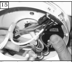
Place and press firmly on the capacitor to stick it to the switch housing. Be sure it is secure.
