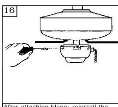
After attaching blade; reinstall the switch housing using the three screws previously removed.
