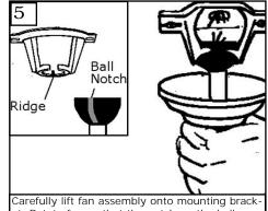
Carefully lift fan assembly onto mounting bracket. Rotate fan so that the notch on the ball engages the ridge in the mounting bracket. This will allow hands-free wiring. For wiring instructions please refer to page 4 step #7.
