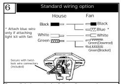
For pullchain controls, follow diagram above. Make sure that all exposed wiring is secured inside wire nuts. Note: Wires from house may vary in color and may not include ground wire. After wiring is conplete, gently push wires into junction box with wire nuts pointing upward. Refer to point 3 of safety tips.
