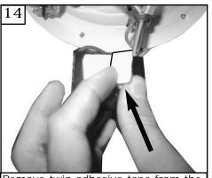
Remove twin adhesive tape from the black capacitor as shown above.
