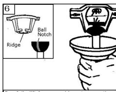
Carefully lift fan assembly onto mounting bracket. Rotate fan so that the notch on the ball engages the ridge in the mounting bracket. This will allow hands-free wiring.
