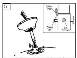
Feed motor lead wires through downrod/canopy assembly and insert downrod into motor yoke. Next, insert clevis pin through yoke and downrod and secure with cotter pin. (see Inset) Tighen both yoke set screws to further secure downrod.
