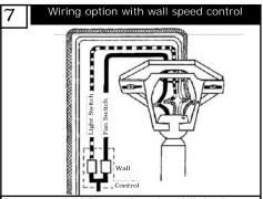
For control of fan and optional light from wall location, follow diagram above. NOTE: A professional electrician is recommended for this type of installation.
