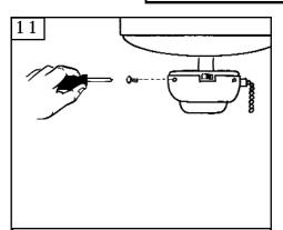
To gain access to the blade bracket attachment holes remove the switch housing cover by unscrewing the three screws. Gently slide the cover off.
