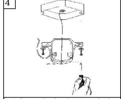
Install mounting brackets to outlet box in ceiling using the screws provided with the outlet box and washers.
