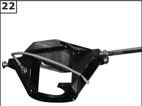
22 Take 4 screws from hardware pack and insert 2 one on each side of bracket to match the L slot screw holes in canopy. Keep 2 screws for later use.
