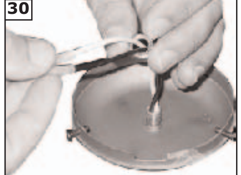
30 Install keeper nut over lead wires.
