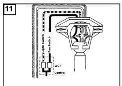
For control of fan and optional light from wall location, follow diagram above. NOTE: A professional electrician is recommended for this type of installation.
