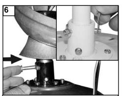
Insert downrod into motor yoke. Next, insert clevis pin through yoke and downrod and secure with cotter pin. (see inset)
