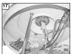
Install switch housing plate by twisting plate with key hole slots into place. Replace screw removed and tighten the 3 screws securely.
