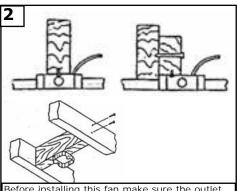
Before installing this fan make sure the outlet box is properly installed to the house structure. To reduce the risk of fire, electric shock, or personal injury, mount to outlet box or supporting system acceptable for fan support. (Mounting must support at least 35 lbs.)
