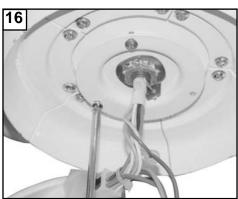
Loosen 2 screws with key slots and remove 1 screw without slot from motor plate and save screw.
