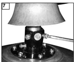
Tighten both yoke set screws to further secure downrod.
