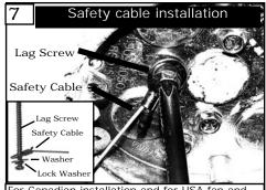
Canadian installation and for USA fan and light kit combinations over 35 lbs, in both flush and downrod mode the safety cable must be installed into the house structure beams using the 3" lag screws provided. Make sure that when the safety cable is fully extended the leadwires are longer than the cable and no stress is placed on the leadwires. stress is placed on the leadwires.
