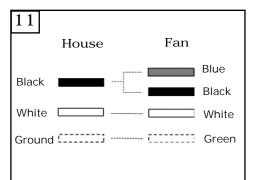
Connect black and blue wire from fan to Black or (Hot) wire from house. Connect White wire from Fan to White (Neutral) wire from house. Connect Ground leads from mounting bracket and downrod to Ground lead from house. Refer to Safety Tips section of
