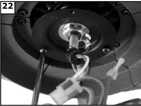
22 Loosen 2 screws and remove 1 screw from motor plate. Save removed screw for use later.
