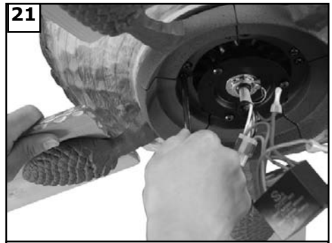
21 Check the motor for plastic shipping stabilizer tabs, and remove them if they are present. Attach blade assembly to motor using the motor screws and washers provided. Tighten screws securely.
