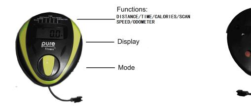
**MODE:** This button cycles through the available Displays and turns the unit ON. Press and hold this button for 3-4 seconds to reset the data values of the monitor.
