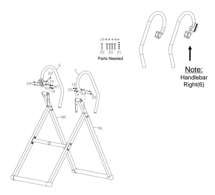
Attach the Handlebars (6) and (7) to the Base Frame Rear (8L and 8R) using 4 Bolts (20), 4 Flat Washers (19), and 4 Nuts (21). Use Bolt (22) and Flat Washer (19) to fix the Right Handlebar (6) to the Base frame Rear (8R).
