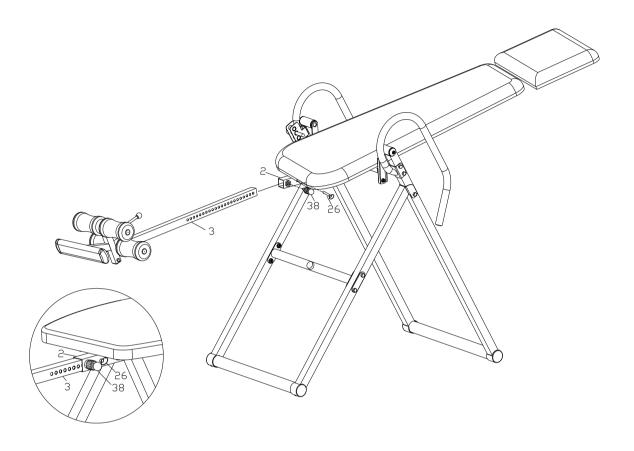
Slide Height Adjustment Tube (3) into Backrest Support Tube (2) and lock into place using Height Adjustment Knob (38), then fully insert the ball pin (26).
