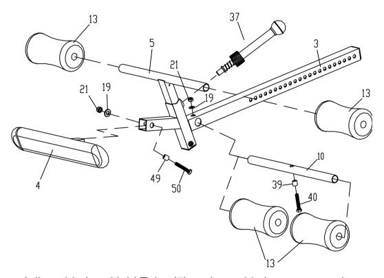
Pull out Adjustable Leg Hold Tube (5) and turn 90 degrees to make sure the holes are on top, then position horizontally as shown. (Part (5) has spring pre-assembled inside Tube which should not be removed.)
