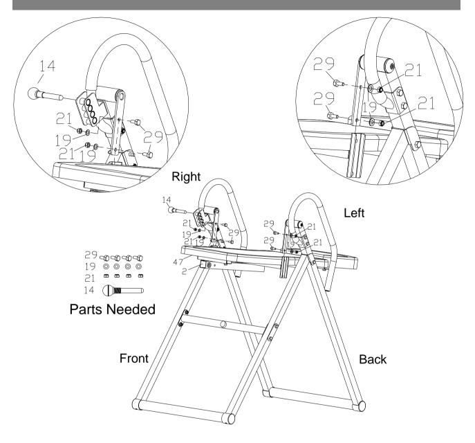
Attach the completed Backrest Pad and Head Pad Assembly to the Base Frame Unit using 4 Bolts (29), 4 Flat Washers (19) and 4 Lock Nuts (21).
