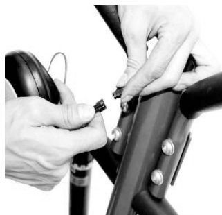
Pull out the wire from the tube and connect with the meter wire.
