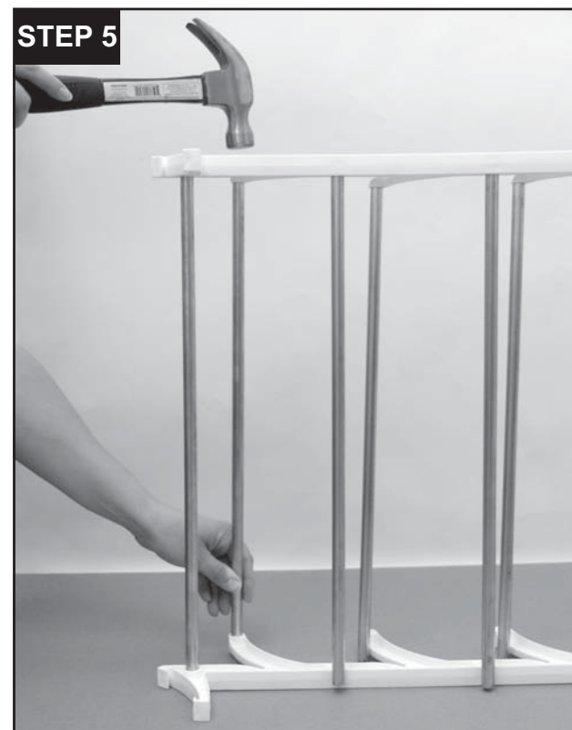
STEP 5: Guide each tube into socket and gently tap to hold in place.
