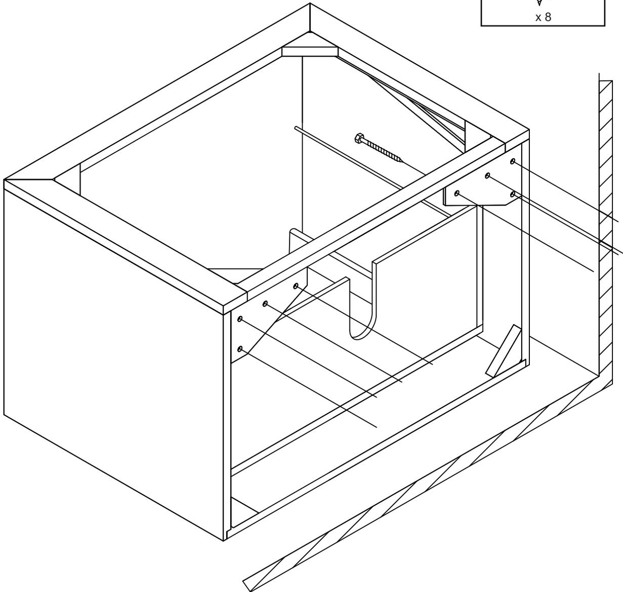
Level the vanity with a leveler and attach the brackets to the 2 x 12 header using screws provided.
