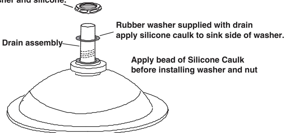
**Place Lavatory face down and apply a bead of silicone caulk to the face of the drain outlet, use plumbers putty to seat the drain in the lav bowl and wrap teflon tape on all threads before joining parts of the drain. The application of the beads of silicone as shown will ensure a leak free installation using metal or plastic drains.**
