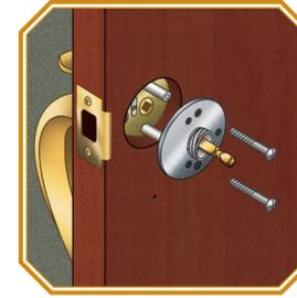
**5** Remove the #10-32 x 1 1/4" truss head screws securing the inside adapter. Remove inside adapter. Discard the adapter and screws.
