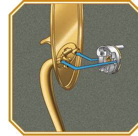
**4** Position the new thumblift cartridge against the handleset, making sure the lugs on the thumbpiece seat into the pockets in the cartridge.
