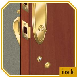
**6** Tighten the #10-32 x 2½" screw. Screw on the 1" round screw cover to the screw cover backplate.
