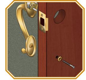
**6a** Supporting the handleset with one hand, unscrew and remove the lower #10-32 x 2 1/2" flat head screw and screw cover backplate. Remove the handleset.
