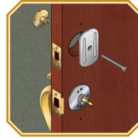
**4** Remove the #8-32 x 2 1/4" flat head screw securing the dummy cylinder adapter to the dummy cylinder. Put the dummy cylinder adapter, dummy cylinder and screw to the side for reassembly later in the installation.
