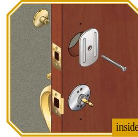
**3** Place dummy cylinder through the cylinder hole in the top of handleset. Thread #8-32 x 2¼" flat head screw through the dummy cylinder adapter and into the dummy cylinder. Tighten all screws.
