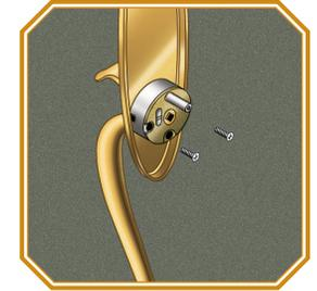
**5** Locate the new thumblift cartridge over the screw posts and secure it with the new 6-32 x 7/16" flat head screws provided. The post on the cartridge should be at the top, and the face of the cartridge should be flush with the surface of the handleset.
