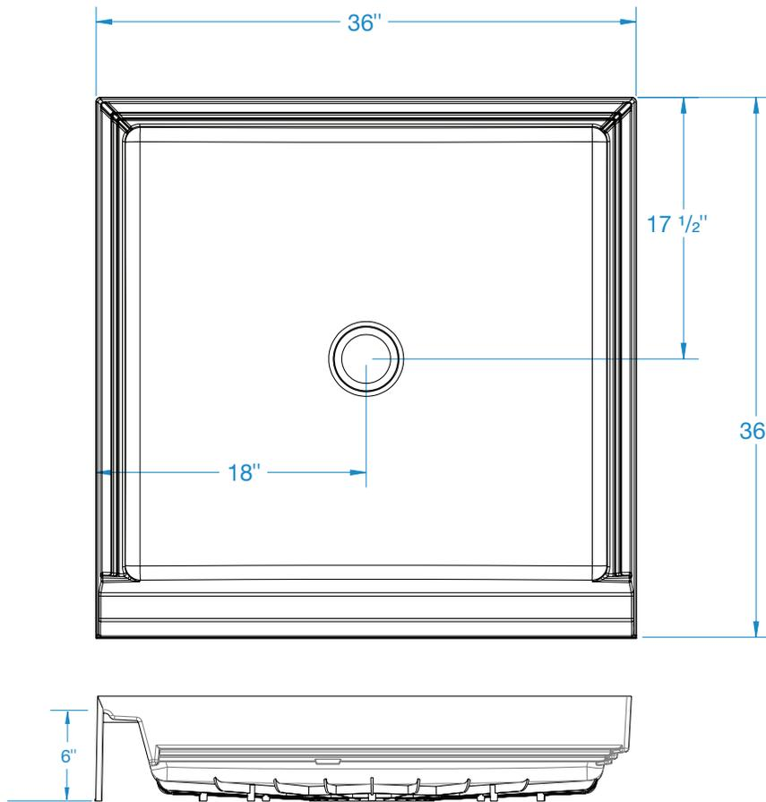
**FEATURES** lbs (kg) Dimensional Tolerance  $\pm \frac{3}{16}$ ". Dimensions needed for site preparation should be measured from the unit. Aquatic assumes no responsibility for preparatory work.
