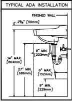
IMPORTANT: These dimensions are nominal and may vary within the range of tolerances established by ASME Standard A 112.19.2 Contact your local building code for approved barrier free measurements.
