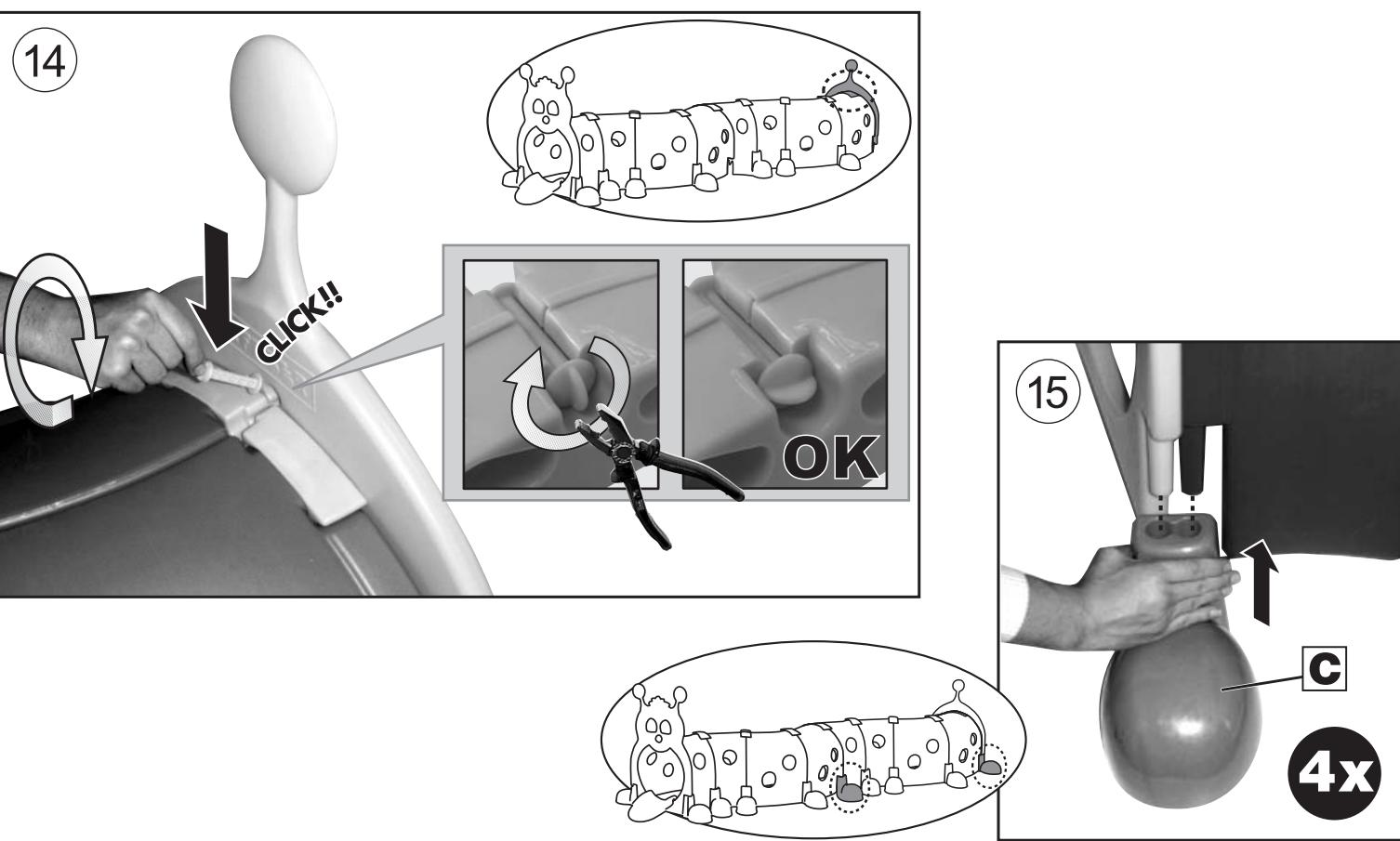
INSTRUCCIONES DE DESMONTAJE • INSTRUCTIONS FOR DISMANTLING • INSTRUCTIONS DE DÉMONTAGE
