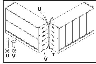
14. Fasten the Piano Hinge(T) to the Right Side(A2) of the Left Unit and the Left Side(G2) of the Right assembled units using 6 Posts(U) and 6 Post Screws(V) as shown.
