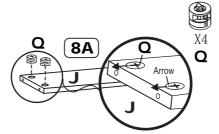
8A. Insert 4 Cams(Q) into the large holes in 2 Dividers(J), using 2 in each. Make sure the arrows on Cams(Q) point toward holes in the closest edge.
