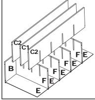
3A. Two Adults Suggested: Carefully lay the unit down on its back. Insert a Middle Shelf(C2) into the bottom slots on the Dividers(F) as shown until fully inserted.
