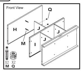
10A. Insert 2 Metal Dowels(M) into the plastic plugs located underneath the Top Shelf(H). Tighten using a Phillips Screwdriver.
