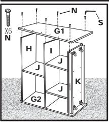
12B. With the unit still on its side, attach Right Side Panel(G1) using 6 Large Hex Screws(N) as shown. Tighten with the Hex Key Tool(S).
