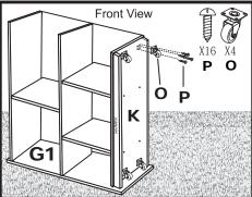
12A. On a carpet or protected surface, lay the unit on the Left Side(G1). Attach 4 Wheel Casters(O) underneath Bottom Shelf(K) using 4 Caster Screws(P) for each caster (16 total). Tighten with a Phillips Head Screwdriver.
