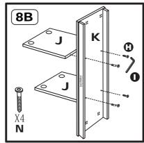
8B. Attach 2 Dividers(J) to the Base(K) with 4 Large Hex Screws(N), using 2 in each as shown. Tighten using the Hex Key Tool(S).
