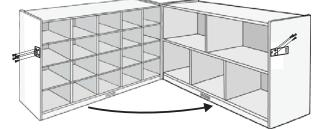
15. Install the Safety Hasp(W) to the outside of the unit using the 7 screws provided.
