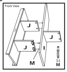
9. Position the Middle Shelf(I) so the attached Metal Dowels(M) enter the holes in the top edge of the 2 lower Dividers(J) as shown. Turn the Cams(Q) with a Phillips Screwdriver until locked onto the Metal Dowels(M).
