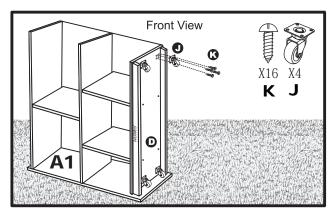
5. **Two Adults Suggested:** On a carpet or protected surface, carefully lay unit onto the Left Side(A1). Attach the 4 optional Wheel Casters(J) underneath the Bottom Shelf(D) using 4 Caster Screws(K) for each caster (16 total). Tighten with a Phillips Head Screwdriver.
