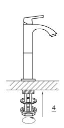
4. PLACE NEW FAUCET IN THE POSITION ON THE SINK. PLACE BRASS RING BETWEEN BOTTOM OF THE FAUCET AND SINK SURFACE. FROM UNDER THE SINK, PUT RUBBER WASHER AND THREAD NUT ONTO THE PIN. TIGHTEN NUT.
