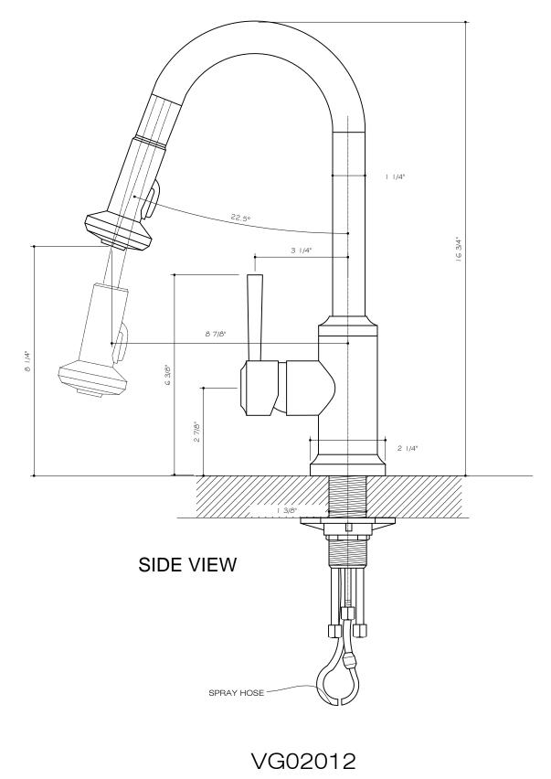
THE MEASUREMENTS IN INCHES ARE ROUNDED TO THE NEAREST 1/8"
