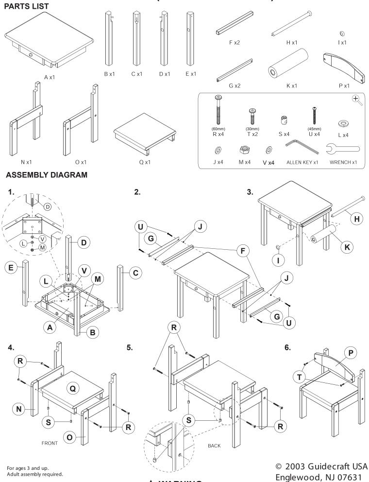
Assembly Note: To ease assembly, do not fully tighten screws during assembly process. After unit is fully assembled go back and tighten all screws.
