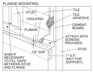
This is done for all three walls of the shower enclosure. In Method #2, a mounting surface is built out flush with the vertical wall of the unit and the same width as the base threshold as shown below.
