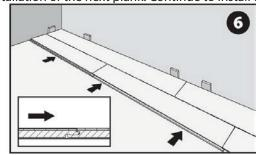
When the entire row is completed, remove all wedges and review the row to ensure there is no gapping and that all locking mechanisms are fully engaged (all planks are perfectly flat). Note: Never hammer planks without using a tapping block or damage to plank edges will occur.
