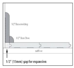
• Above, on, or below grade: Flooring must be installed by floating planks over a wooden or concrete subfloor
