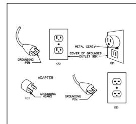
warning: This heater has a voltage rating of 120 volts. The cord has a plug as shown in A. An adapter as shown in C is available for connecting three-blade grounding-type plugs to two-slot receptacles. The grounding lug extending from the adapter must be connected to a permanent ground such as a properly grounded outlet box. The adapter should not be used if a three-slot grounded receptacle is available.
