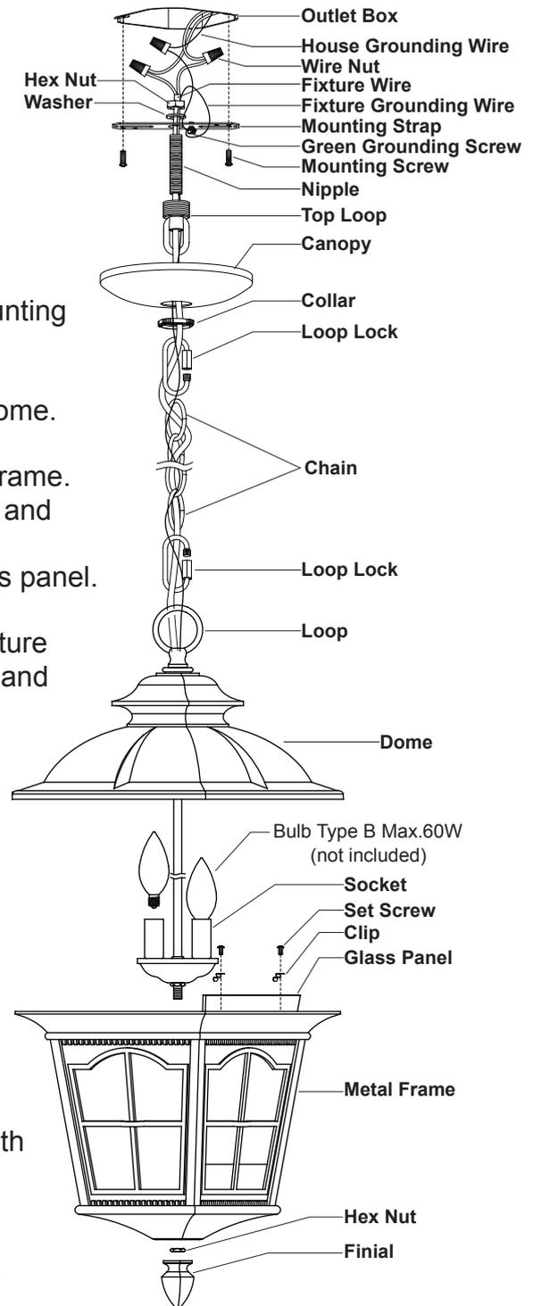
**CAUTION: With silicone caulking compound, caulk completely around where back of canopy meets with the ceiling surface to prevent water from seeping into the outlet box.**
