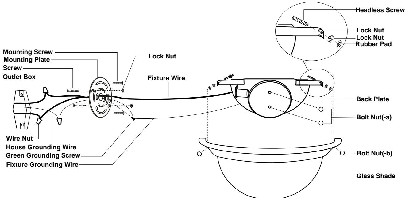
1. Unscrew bolt nuts(-a) from the back plate, and remove the mounting plate.
