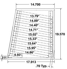
\*MAXIMUM DEPTH OF EQUIPMENT SPACE FROM OUTSIDE FRONT RAILS TO INSIDE REAR RAILS. (±.060) .70" EXTRA SPACE IS AVAILABLE TO THE BACK OF THE CABINET FOR ALL BUT THE BOTTOM TWO SPACES.
