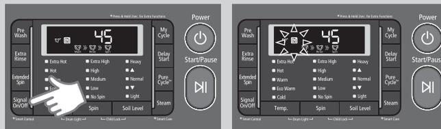
Once the Wi-Fi icon is displayed press and hold the "Signal" for 3 seconds. The Wi-Fi icon will stop blinking. The machine is now ready to run the device certification.
