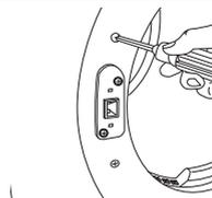
6. Remove the two screws from the holder lever.
