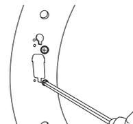
8. Remove a screw from the door hinge.
