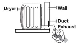
2. Use a 4" diameter rigid metal duct. Tape all joints, including at the dryer. Never use lint-trapping screws.
