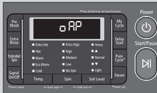
When the network is setup the unit will display "Transfer complete". After the transfer is completed select "Confirm". The unit will then display "oAP". The phone is now connected to the machine through the network.
