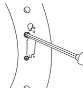
5. Remove the two screws from the opposite side of the door hinge.
