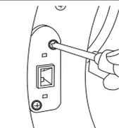
7. Reassemble the two screws on the inside holes.
