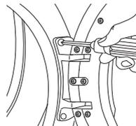
4. Remove two screws from the frame front.
