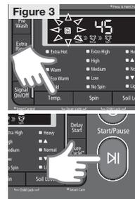
3. Once the "AP" is displayed you need to turn the knob counter clockwise until "PS" is displayed. After the "PS" is displayed press the Start/Pause button.
