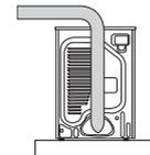
4. Clean all old ducts before installing your new dryer. Be sure the vent flap opens and closes freely. Inspect and clean the exhaust system annually.
