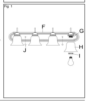
NOTE: INSTALL THE GLASS ASSEMBLY AFTER THE FIXTURE IS HUNG.
