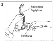
Connect the water supply lines. Before connecting the supply lines, apply pipe joint compound to the threads on the inlet shanks and shut off valves.
