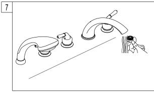
7. Remove the aerator before turning on your new faucet for the first time. Allow both hot and cold water to run for one minute. Replace aerator.
