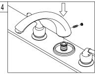
4. Place spout into spout hub. Complete installation by inserting set screw hole cover into access hole in back of spout.
