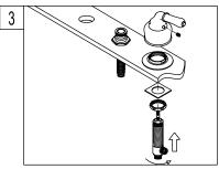
3. Hold the escutcheon of handle in proper position. Make sure that the top of the faucet handles is 5/8" above the top of the sink. Mount the metal washer and locknut from underneath the sink. Then reposition escutcheon as necessary to a desired height.
