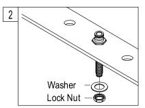
To keep spout from rotating after installation, screw brass pin into spout base. Then place spout escutcheon on over spout tube hub. Place mounting washer on spout shank and attach with spout shank locknut.
