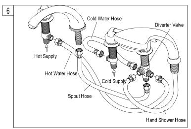
6. Connect the flexible tubes from the supply shank side port to the diverter valve. Also reattach the supply lines, turn on the water supply, and check for leaks.
