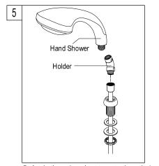
5. Apply thread sealant tape to threaded end of hose. Thread hose from top through the hand shower holder, and install tightly to the diverter valve. Attach hand shower.
