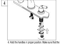
4. Hold the handles in proper position. Make sure that the top of the faucet handles is 5/8" above the top of the sink. Mount the metal washer and locknut from underneath the sink. Than reposition escutcheons as necessary to a desired
