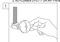
Shut off hot and cold water supply under sink.
