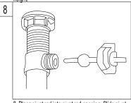
8. Place pivot rod into pivot rod opening. Slide pivot nut over pivot rod and thread it on the drain body. Tighten firmly.
