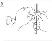
10. Guide the pivot rod through one of the holes on the lift rod strap and secure it with the spring clip. Then adjust the height of the lift rod by resetting the clevis screw.
