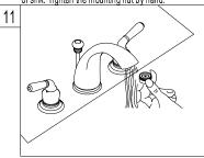
11. Remove the aerator before turning on your new faucet for the first time. Allow both hot and cold water to run for one minute. Replace aerator.
