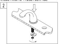
Install new faucet spout through the center hole of sink. Place mounting washer on spout shank and attach with spout shank locknut.
