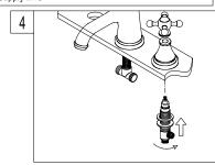
4. Hold the handles in proper position. Make sure that the top of the faucet handles is 5/8" above the top of the sink. Mount the metal washer and locknut from underneath the sink. Than reposition escutcheons as necessary to a desired height.
