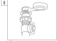
Thread mounting nut and bottom gasket onto drain body. Wrap top threaded end of the drain body with plumbers' tape.
