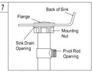
7. Install drain body up through the drain opening and reattach the flange onto drain body, holding the drain body in position with pivot rod opening facing the back of sink. Tighten the mounting nut by hand.
