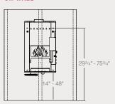
Must mount to a minimum of one (1) wall stud.
