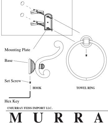
1. Hold base of the product on desired wall location and lightly mark outline of base. Place mounting plate in vertical position, with rounded edge facing up at center of marked outline and mark a dot at center of each of it's two slotted holes.
