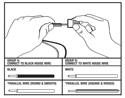
\*Note: When parallel wire is used, the tracer wire is square shaped or ridged and less tracer wire is round in shape or smooth
