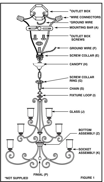
WARNING: TO REDUCE THE RISK OF FIRE, ELECTRIC SHOCK OR PERSONAL INJURY, MOUNT TO OUTLET BOX OR SUPPORTING SYSTEM ABLE TO SUPPORT THE WEIGHT OF THE FIXTURE.
