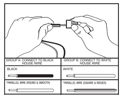
\*NOTE: When parallel wire is used, the tracer wire is square shaped or ridged, and the less tracer wire is round in shape or smooth. (Seen best when viewed from wire end.) To separate wires, grasp the ends of each wire and pull apart.
