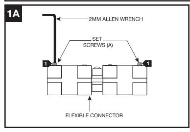
1 Clear the connector open ends by backing out (DO NOT REMOVE) the two set screws (A) with the provided 2MM Allen wrench.
