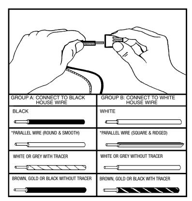
\*Note: When parallel wire is used, the tracer wire is square shaped or ridged and less tracer wire is round in shape or smooth. (Seen best when viewed from wire end.) To separate wires, grasp the ends of each wire and pull apart.
