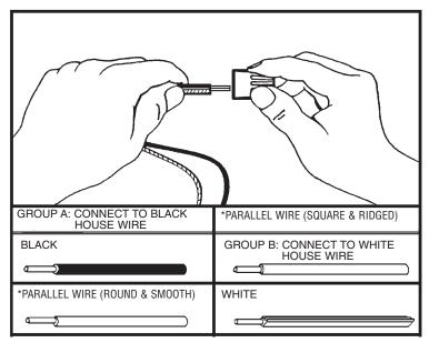
\*Note: When parallel wire is used, the tracer wire is square shaped or ridged and less tracer wire is round in shape or smooth.
