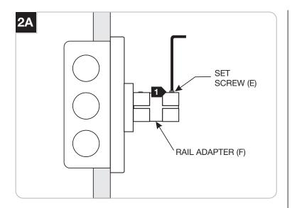
Back out (DO NOT REMOVE) the set screw (E) with the 2MM Allen wrench to clear the rail adapter (F).
