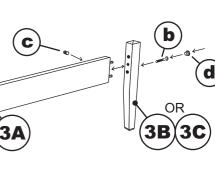
Attach the Legs (3B or 3C) to Mid Rail(3A),using JCB M6X 60mm (b) and Barrel Nut (c). Tighten with the Allen Key (e). Lastly push in Wood Button (d) as shown.
