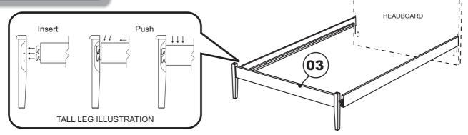
Attach the other end of the Long Rails to the Footrail (03) using bed hook as shown.
