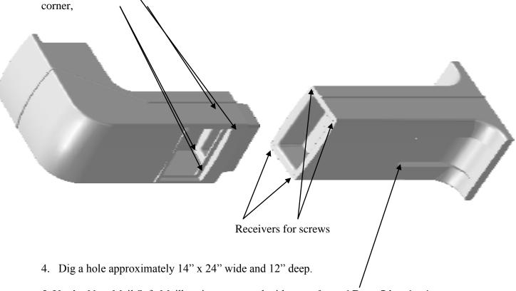
5, You're New Mail Safe Mailbox is constructed with a pre-formed **Bury-Line** that is pre measured to the correct installation height. (38" to 42") and does not need any additional material to make it solid.
