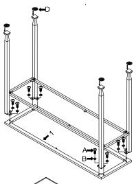
3. Turn the unit upside down, put the glass pads (C) on the frame, then put on (5) top glass and insert (6) glass shelf as shown.
