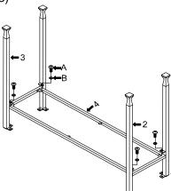
2. Using screw (A) & (B) to assemble the top frame (1) and the legs as shown then add the foot pad (D) onto the end of leg.
