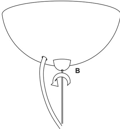
1. Carefully unpack parts. Remove the Canopy (A) from the Mounting Plate by unscrewing the Retainer (B). Fully remove the Retainer from the threaded nipple, then pull the canopy from the Mounting Plate.
