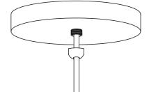
6. Lift the canopy up to the ceiling and tighten with the Retainer, but do not overtighten.
