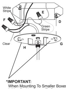
When Mounting To Smaller Boxes, It May Be Necessary To Secure Using These Mounting Holes.
