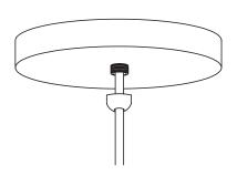
6. Lift the canopy up to the ceiling and tighten with the Retainer, but do not overtighten.
