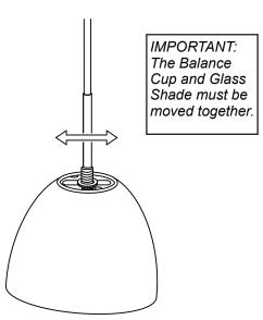
C. Slide both the Glass Shade and the Socket Assembly into a new position along the slot in the Balance Cup that will level the Glass Shade. It may be necessary to loosen the Knurled Nut during this step.
