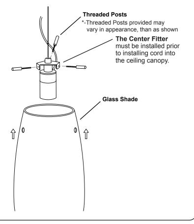
All electrical connections and the installation of this fixture must be in agreement with local codes, ordinances or the NEC (National Electric Code) or CEC (Canadian Electrical Code).
