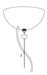
6. Replace the Canopy as shown and secure with the Retainer. Tighten the Retainer enough to hold the Canopy to the ceiling but do not overtighten. The cord can now be shaped by positioning the Cord Rings (J) along the cable as desired.
