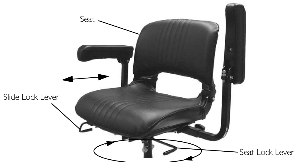
FIGURE 7.3 Adjusting 90° Seat Swivel
